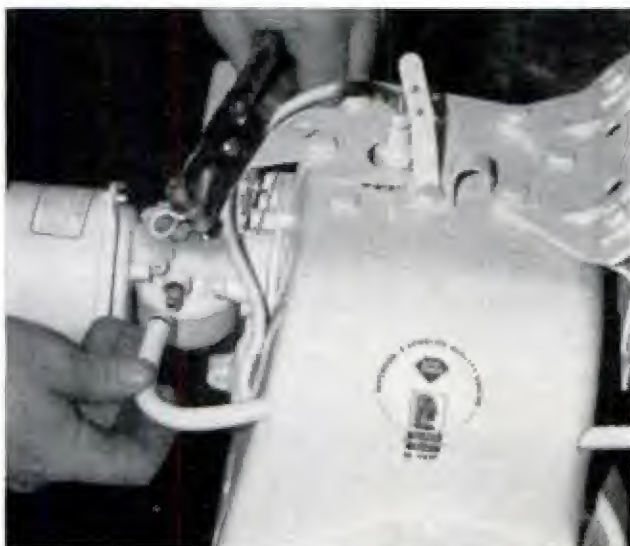
FUEL STOPPAGE AT CARBURETOR? Unhook fuel line at carb. Fuel flows? It's getting to, not through, carb MARCH 1971
